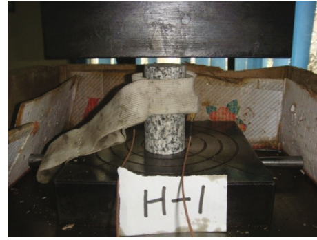
FIGURE 1: Installation of acoustic emission sensor.
