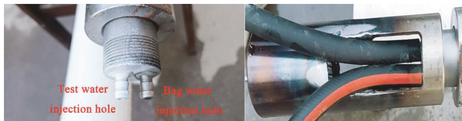
FIGURE 13: Water injection hole and tail connector of a double-end water shutoff.
