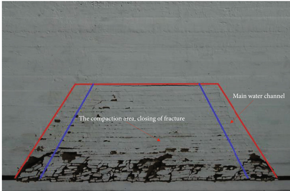
FIGURE 5: Main water channels in the fracture zone.
