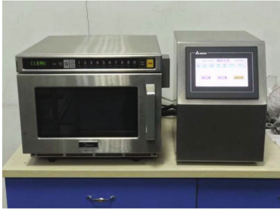
FIGURE 1: The modified commercial microwave oven.
