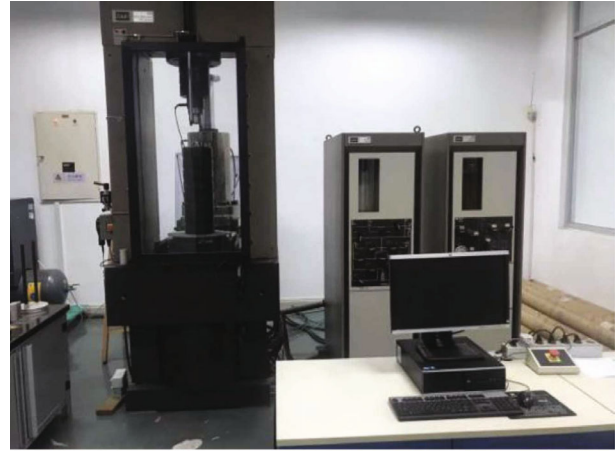
FIGURE 2: The MTS815 mechanical testing machine of rocks.
