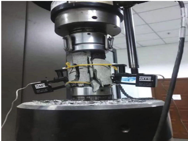
FIGURE 9: Uniaxial compression effect of the basalt sample.
