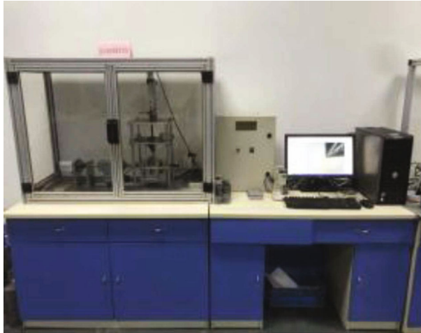
(a) Abrasion servo tester of rocks
