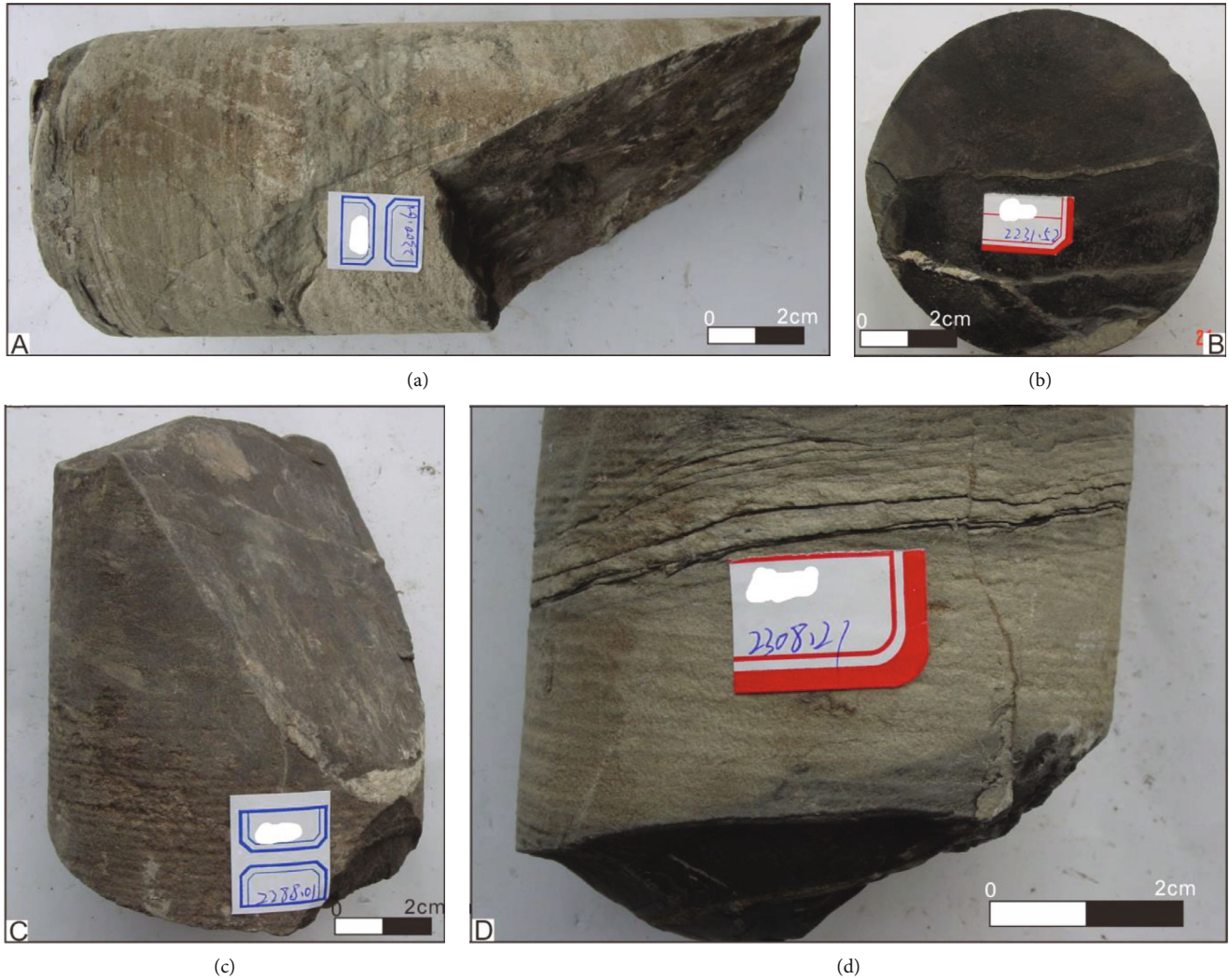
FIGURE 3: Fracture development characteristics of the Subei Basin. (a) Shear fractures developed in mudstone of Well S10, filled with mud, 2300.61 m. (b) Shear fracture developed in mudstone of Well J2, filled with calcite, 2231.52 m. (c) Shear fracture developed in mudstone of Well S10, unfilled, 2288.01 m. (d) Tensile fracture developed in mudstone of Well S10, 2308.21 m. Due to the requirement of confidentiality of oilfield data, we did not display the actual well name.
