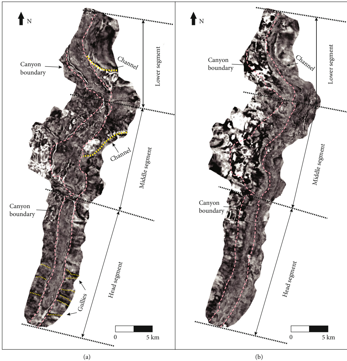
FIGURE 12: (a) Coherence slice along the surface 100 m below flattened SB1. The gullies and channels display a dark-coloured coherence pattern, and the canyon fill deposits exhibit a grey-coloured coherence pattern. (b) Coherence slice along the surface, which is 100 m shallower than flattened SB1. The progradation of the platform shows a grey-coloured coherence pattern with convex-westward planform geometries, as visible in plan view. See the position in Figure 4.
