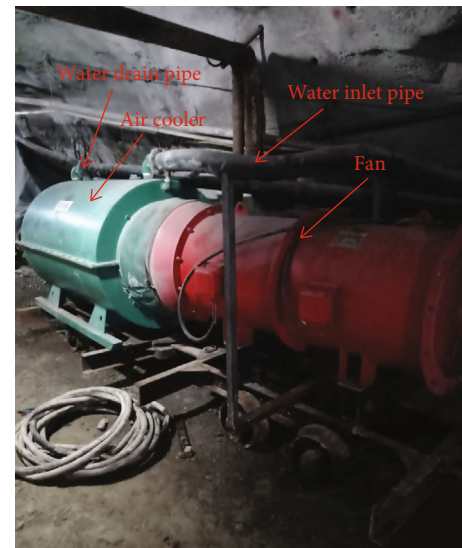
FIGURE 13: Equipment installation drawing.
