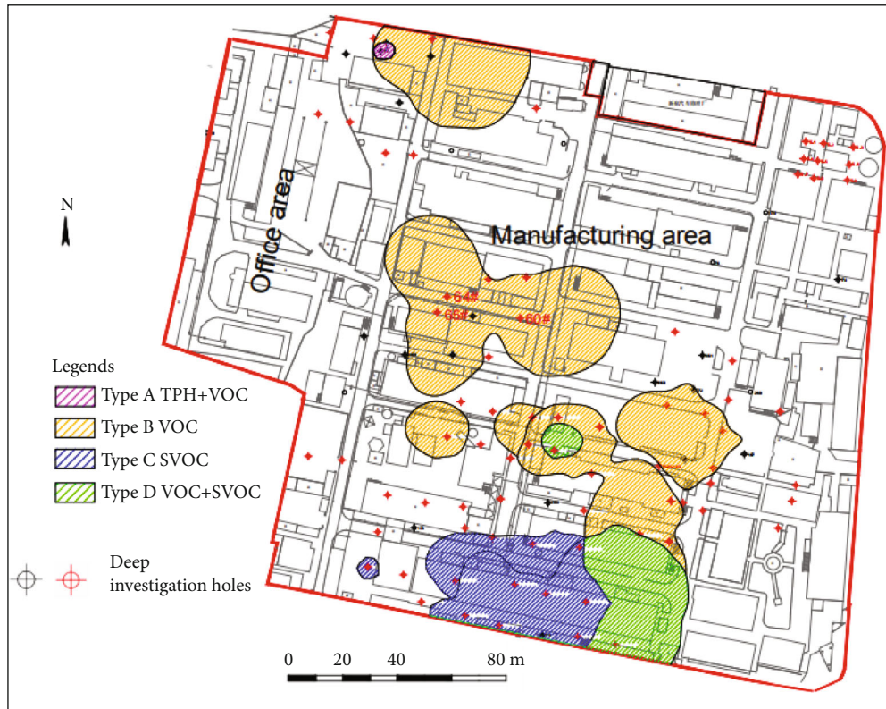
FIGURE 4: Factory plan and contaminant distribution.
