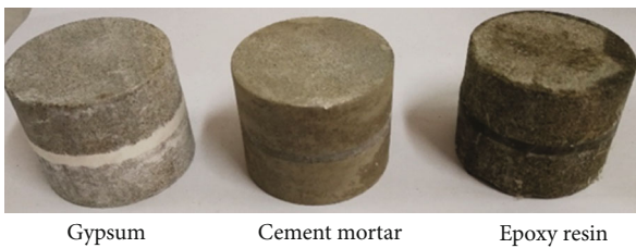
FIGURE 10: Prepared specimens of different joint materials.
