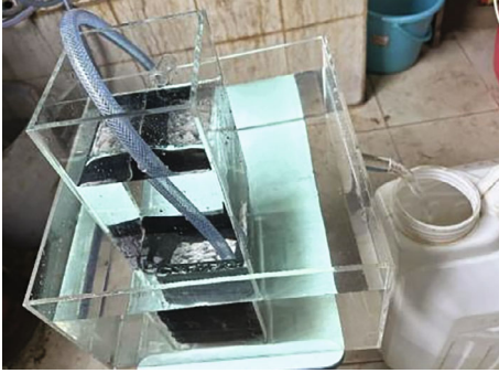
FIGURE 5: Ecological pervious concrete permeability test process.
