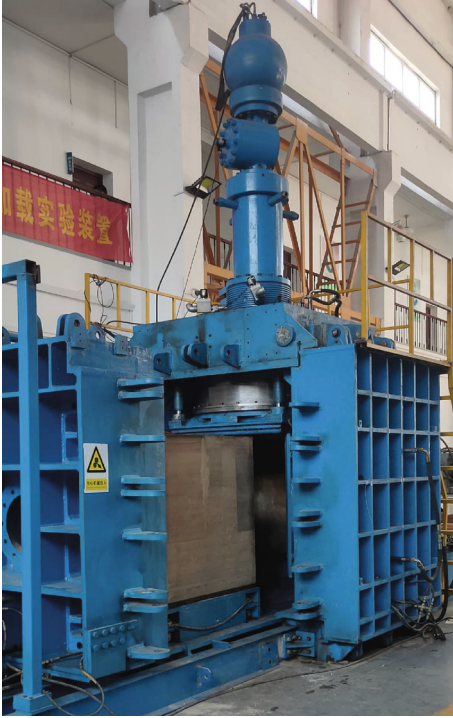
FIGURE 1: Deep-cavern ground-shock disturbance loading system.
