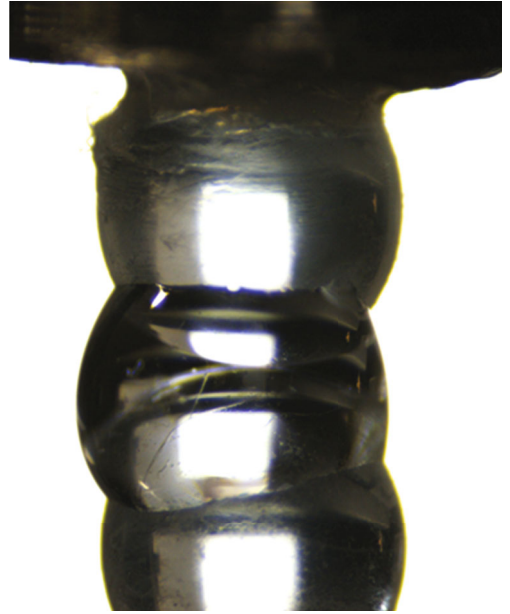
FIGURE 7: Profile of liquid bridge when the Y-L equation is not suitable.
