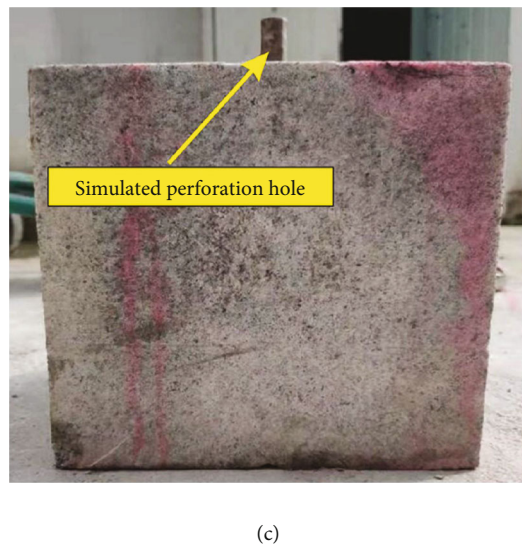
FIGURE 1: Triaxial hydraulic fracturing platform and sample preparation: (a) triaxial hydraulic fracturing platform; (b) schematic diagram of fracturing sample; (c) prepared rock samples.
