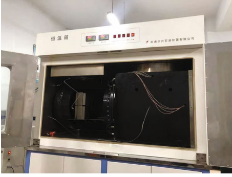
FIGURE 2: The true triaxial hydraulic fracturing equipment and test process.
