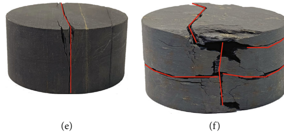
FIGURE 17: The stress-displacement curve of dry and saturated shales: (a) parallel bedding shales without \text{LN}_2 preconditioning; (b) parallel bedding shales after \text{LN}_2 preconditioning; (c) vertical bedding shales without \text{LN}_2 preconditioning; (d) vertical bedding shales after \text{LN}_2 preconditioning. The failure pattern of shale in the Brazilian disc test: (e) parallel bedding shale; (f) vertical bedding shale.
