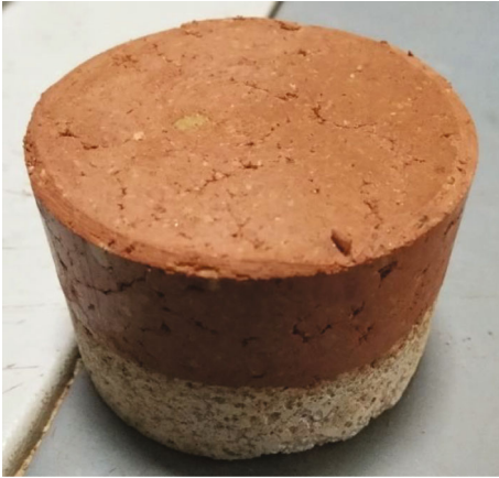
FIGURE 3: Red soil-mortar plate interfacial sample at unfrozen condition.
