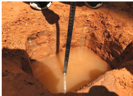
FIGURE 16: Field seepage test using test pit method.
