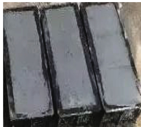
FIGURE 4: Test specimens for dynamic modulus of elasticity. 24 h, 30 h, 36 h, 42 h, and 48 h, respectively, in two curing chambers.
