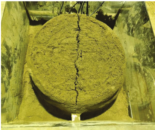
FIGURE 15: The moisture dispersion morphology after the experiment.
