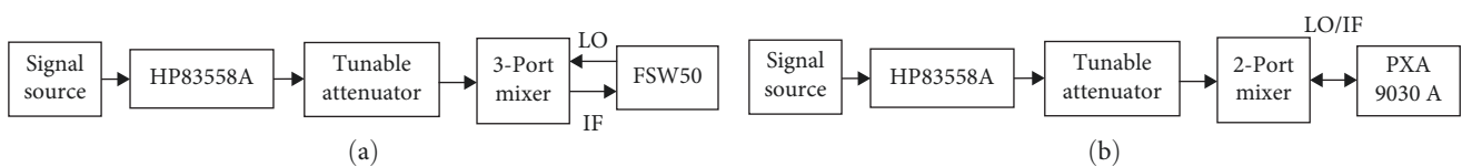
FIGURE 11: Test bench of (a) 3-port mixer and (b) 2-port mixer.
