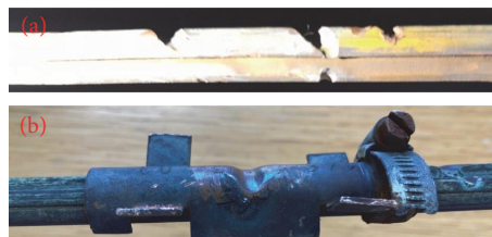
FIGURE 29: Catenary wire (a) and saddle (b) having been worn by stainless steel dropper loop.
