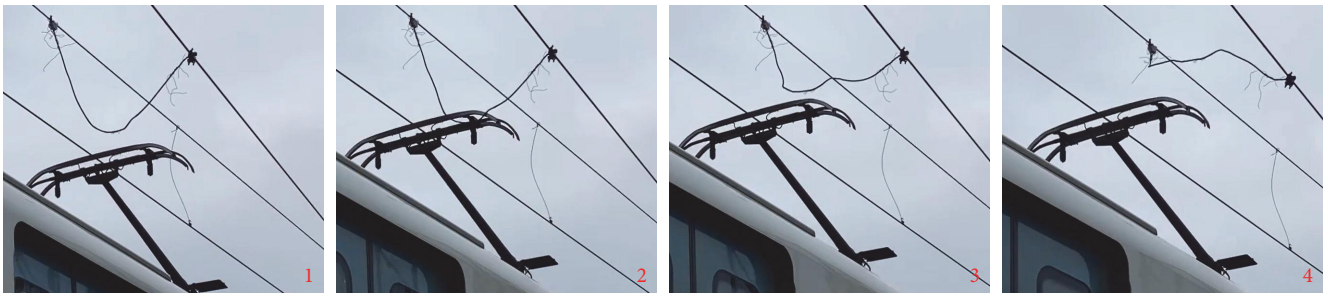
FIGURE 44: Loose jumper hits passing pantograph, 1 → 2 → 3 → 4.
