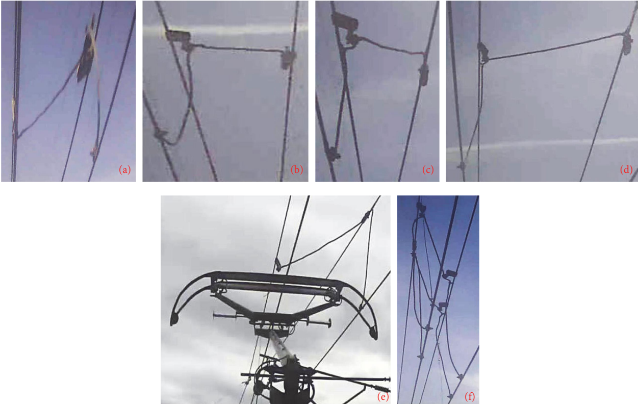
FIGURE 42: Tight potential-equalising (a–e) and full-drape (f) jumpers.
