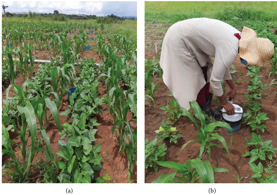
FIGURE 5: (a) Installed pvc chamber/collar and (b) soil CO 2 chamber to measure CO 2 emission rates.
