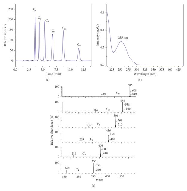
FIGURE 3: (a) LC chromatogram, (b) UV spectrum, and (c) mass spectra of PFCA-DCA derivatives.
