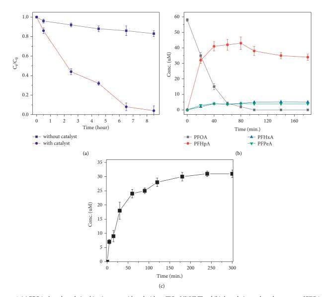
FIGURE 4: (a) PFOA photodegradation kinetic curves with and without  $TiO_2$ -MWCNT and (b) degradation and product curves of PFOA in the presence of  $BiOI_{0.8}F_2$  at pH 6.0 and 25°C. (c) Degradation and product curves of transformed PFOA from PFOSA in the presence of 0.2 M NaOH and 50 mM potassium persulfate.
