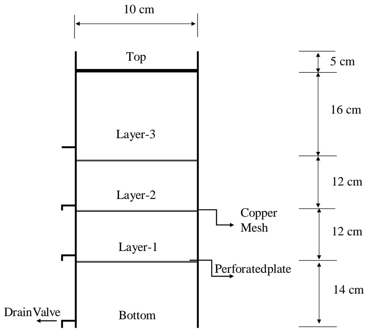
**Figure S1 Home Made Filter for Adsorption**
