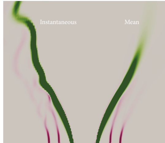
FIGURE 19: Snapshot of instantaneous and mean G value contour behind the bluff body (green, positive; purple, negative; and gray, zero).
