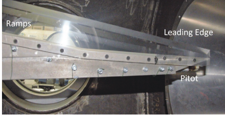
FIGURE 7: Pitot pressure tubes at the leading edge of the compression ramps.
