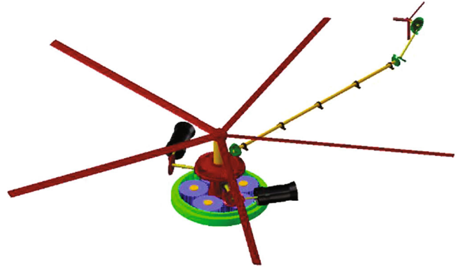
FIGURE 1: The structure diagram of the study helicopter transmission systems.
