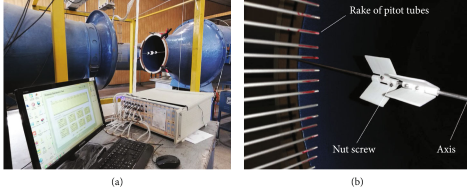
FIGURE 5: (a) Test section, traverse mechanism, and model located on the ring-shaped stand. (b) The rake of Pt probes and splitting airfoils arrangement (close-up).
