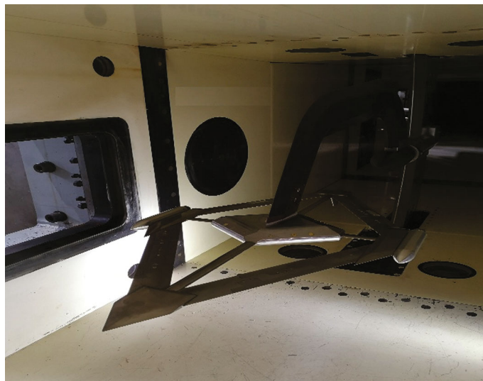
(b) The 60° model of the wind tunnel test
