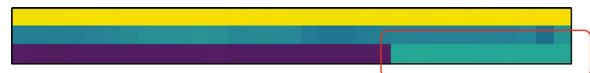
FIGURE 14: State image visualization for the records in Figure 13; width of the image corresponds to the time window (30s), and the 3 rows (from top to bottom) indicate normalized airspeed, AOA, and sideslip angle, respectively; the sideslip drift fault is marked with a red box.
