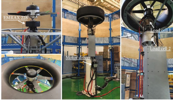
FIGURE 2: The 40% scaled-down ducted fan model and the configuration of the test stand.
