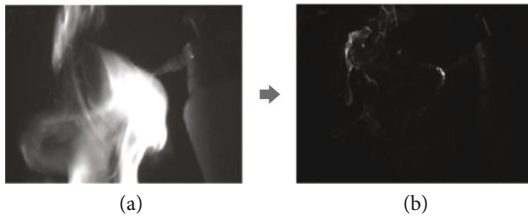
FIGURE 3: Example of a frame measured in different conditions: (a) frame measured with no mechanical shutter; (b) frame measured with a mechanical shutter.
