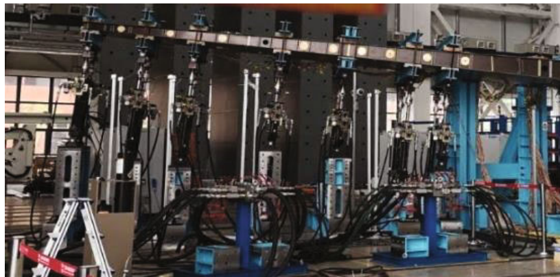
FIGURE 15: Static load experiments of wing structures.
