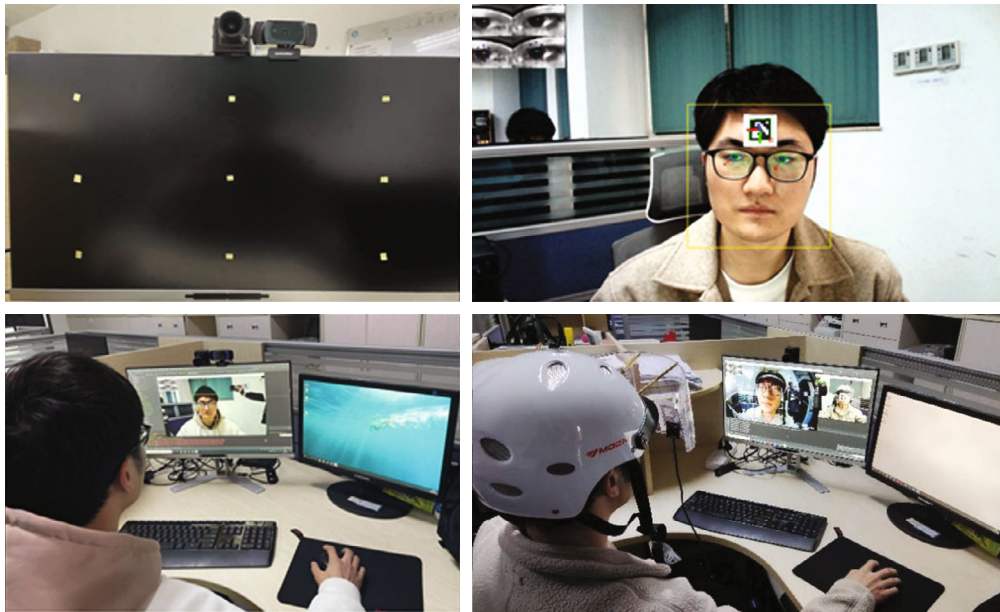
FIGURE 8: Gaze estimation under lab environment. Upper left: nine markers on the screen. Upper right: a subject sat in front of a screen and looked at a marker on the screen. Lower left: the eye feature points are extracted from the webcam and 3D gaze direction is estimated. Lower right: the eye feature points are extracted from the proposed HMD helmet and 3D gaze direction combined with helmet orientation is estimated.
