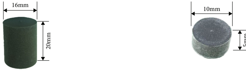
(a) Specimen for the low and medium strain rate uniaxial compression tests (b) Specimen for the high strain rate uniaxial compression tests
