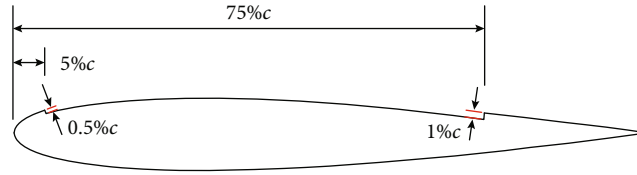
FIGURE 6: Profile of a CFJ-based rotor showing the positions and heights of the two slots.
