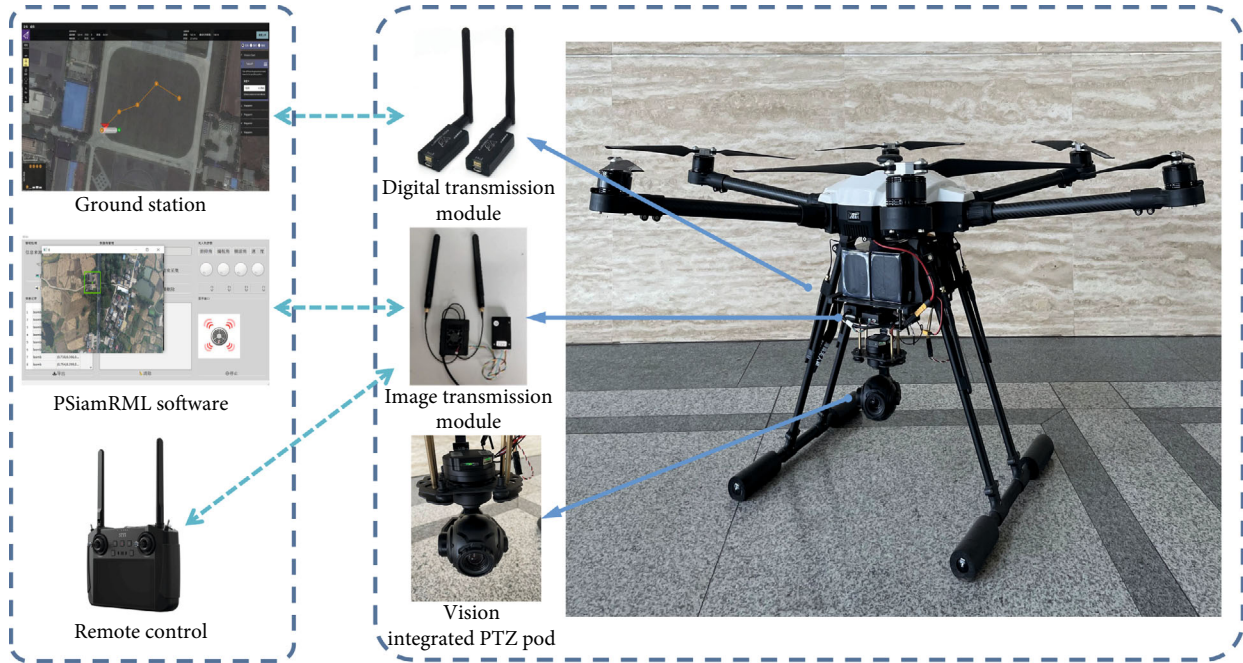
FIGURE 9: UAV visual localization test system.
