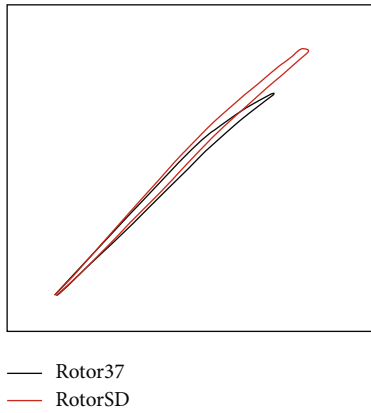
FIGURE 1: Comparison of the geometry of the two rotors at 90% span.
