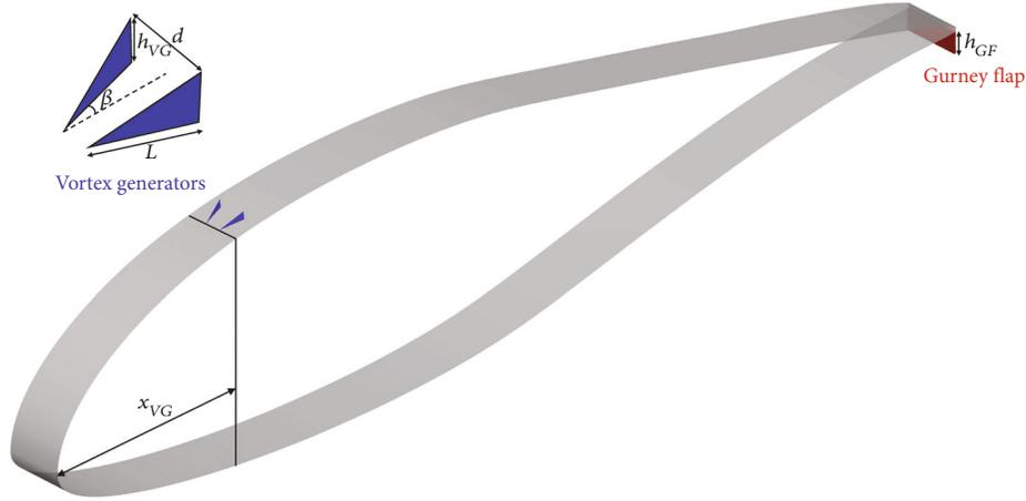
FIGURE 1: Schematic diagram of the A821201 wing equipped with VGs and GF.
