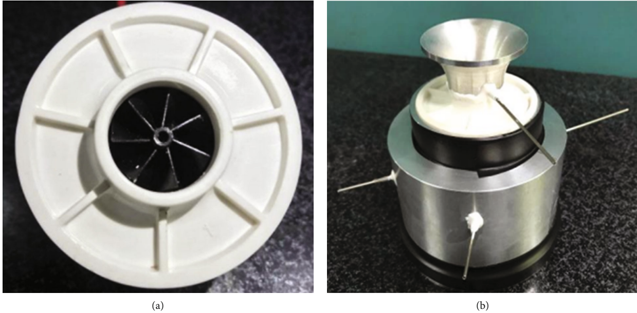
FIGURE 5: (a) The microcentrifugal compressor used in the experiment; (b) the complete experimental setup consists of a trumpet-shaped intake, throttle plate, and pressure tubes.
