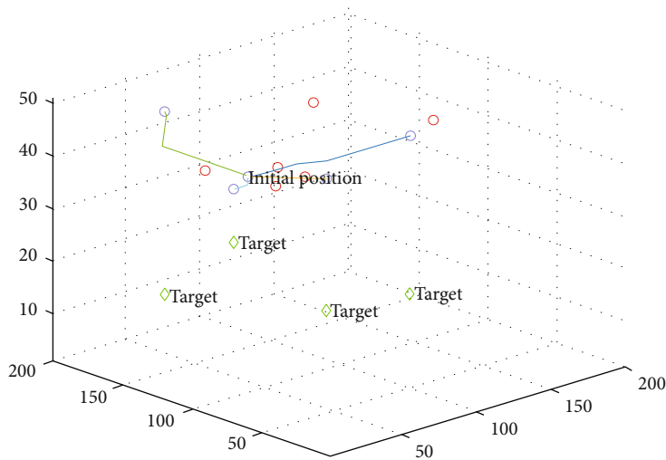
FIGURE 7: UAV swarm path planning via the optimal A* algorithm in the 3D environment.
