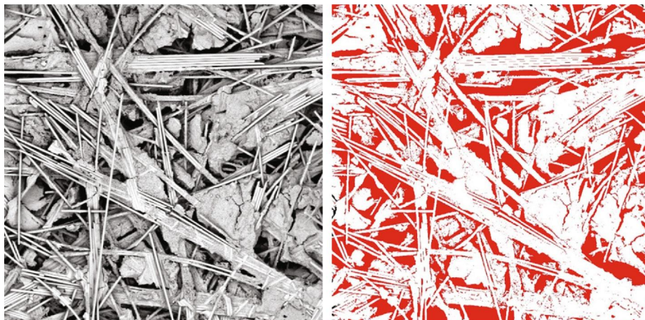
FIGURE 16: Micron-scale pore image and pore labeling map on the back of layer A1.
