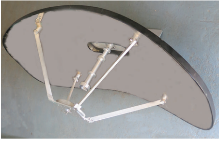
FIGURE 7: Photograph of ring-focus elliptical beam antenna.
