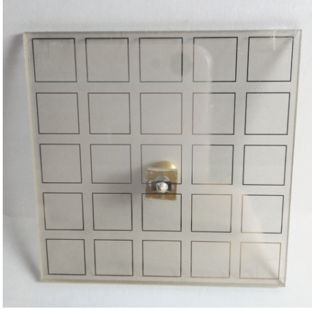
FIGURE 5: Overall view of the fabricated proposed antenna.
