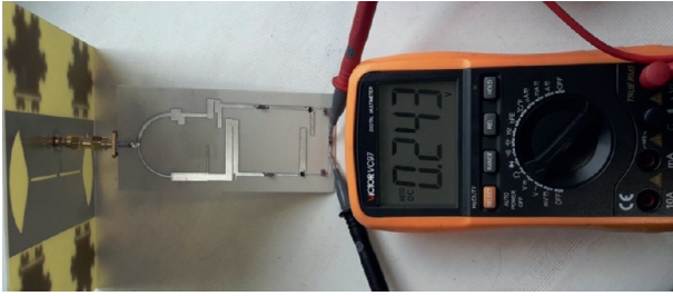
FIGURE 16: Rectenna measurement in a typical indoor laboratory ambience with a voltage meter.
