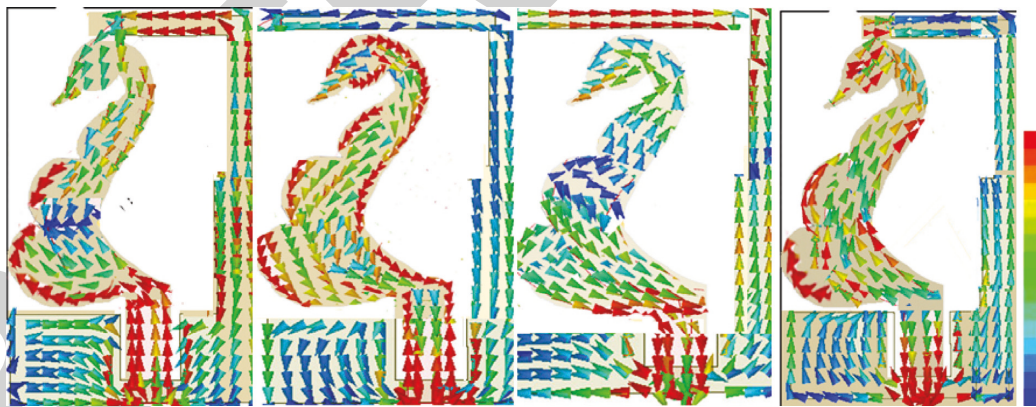
FIGURE 4: Vector current distribution at 5.25 GHz. (a) 0°, (b) 90°, (c) 180°, and (d) 270°. (e) Red indicates the highest peak power, and blue indicates the lowest peak radiation with arrow direction showing flow direction (left to right fig counting).
