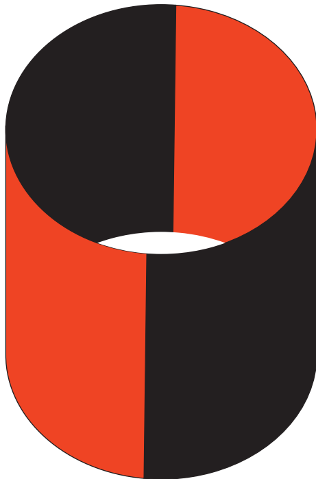
FIGURE 14: Structure of a single-layer two-pair ( a = 1, b = 2 ) electret thin-film mechanical antenna.
