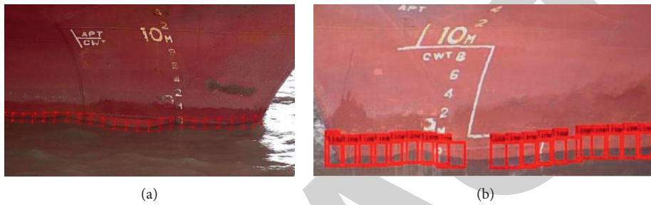
FIGURE 4: (a) Marked image by YOLOv3. (b) Detection image of waterline by YOLOv3.
