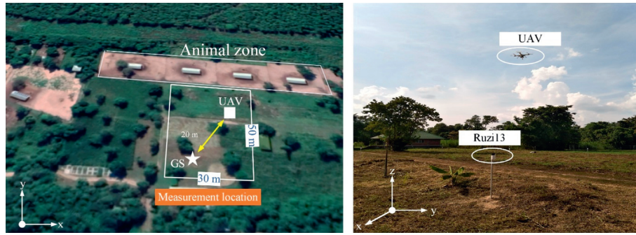
FIGURE 5: Top view of the measurement location and side view of the example test: UAV trajectory at 5 m altitudes in the Ruzi farm.
