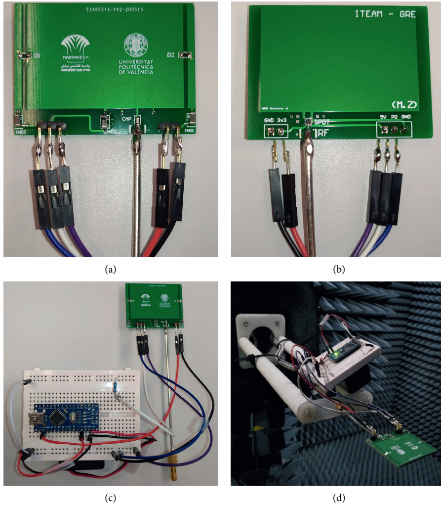
FIGURE 12: Final antenna prototype: (a) top view; (b) bottom view; (c) antenna with bias platform; (d) antenna in anechoic chamber.
