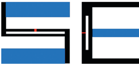
FIGURE 12: Inductive structures in “S” and “E.”
