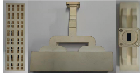
FIGURE 8: Photograph of the fabricated 2 \times 8 array.
